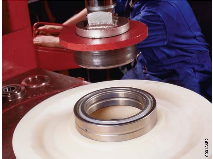
Figure 4 Mounting with control of force and travel
