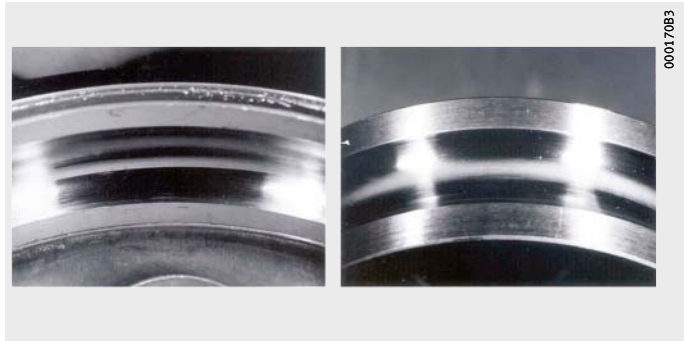
Figure 3 Marks on raceways
