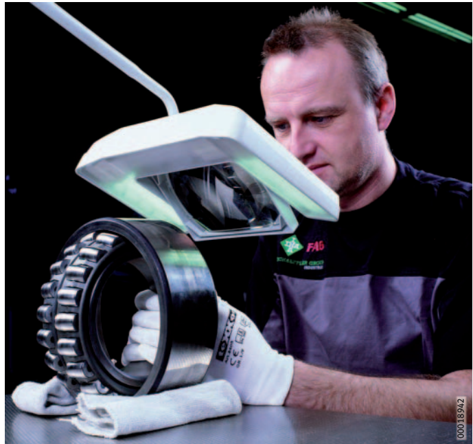
Figure 15 Bearing examination by Schaeffler reconditioning specialists
